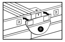
Use threaded holes on elevate kit to attach and secure 6 legs. To return base to it's original height. REMOVE ONE SECTION OF THE 3-IN-1 LEG.
