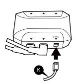
With both bases in FLAT position, connect each base tothe other by inserting each control box slot labeled sync. NOTE: If using 3-in-1 legs, BOTH bases need to be converted to the 3-in-1 to maintain consistent deck height
