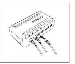
Plug in elevation motor cable into control box's port labeled "tilt motor" (marked in vellow).
