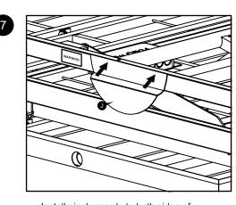
Install pinch guards to both sides of elevation kit (as shown), be sure to install the guards next to the label (not over the label) as per the arrows indicated on the warning labels.
