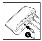
With both bases in FLAT position, connect each base to the other by inserting SYNC CABLE into each control box slot labeled sync.
