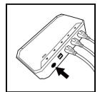
Double click the PAIR button on the control box (light will turn blue during the pairing process).
