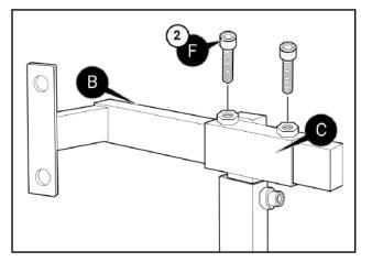
Insert bracket (B) into bracket (C) and lightly secure with two bolts (F).
