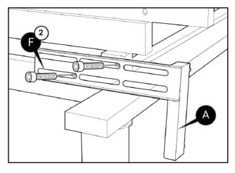
Raise the head of the base to the full upright position. Find the two threaded headboard bracket holes on the frame of the base. Align bracket (A) with the two threaded headboard bracket holes. Lightly secure bracket (A) with two bolts (F).
