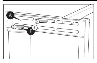
Raise the head of the base to the full upright 1 position. Find the two threaded headboard bracket holes on the frame of the base. Align bracket (A) with the two threaded headboard bracket holes. Lightly secure bracket (A) with two bolts (F).
