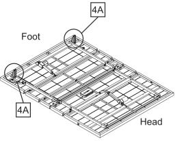
Attach Elevation Kit onto Foot End Angle Bracket
