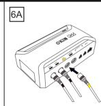
Connect the elevation motor wire to the control box of adjustable base. The wire and control box are color coded. Match YELLOW colors to ensure proper connection.
